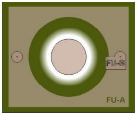
When the white paint has dried sufficiently apply the "B" mask using the registration disks for guidance.
