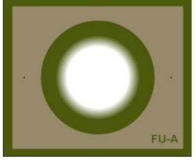
Apply white paint to the centre of the mask to a diameter slightly large than the disk of the "B" mask.
